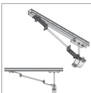
Mounting example Joint angle with bracing
